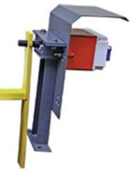
Two (2) downcast arms connected to an electrical switch detect belt misalignment in either direction before damage occurs to the belt or conveyor structure.
