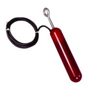
The CTS 600 BCD blocked chute detector is a tilt-type switch, which is mounted inside the chute to monitor any blockage in the material conveyed. Should material start to build up due to a blockage, it will lift the sensing rod, tilting the switch; any tilt to the switch above 15 degrees will cause one of the steel-encapsulated switches to open. This unit provides a relay interface between a tilt-type probe and the conveyor control system.
