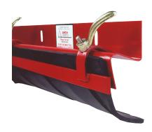
Flexiskirt sealing systems utilize directionally grooved rubber to force fines back into the bulk flow. Recommended for very dry, dusty materials, this design takes advantage of the rubber's natural flexibility to seal the belt by conforming to the belt surface. Able to withstand temperatures of up to 150°F, Flexiskirt seal conforms to the belt's dynamics with minimal friction as it adapts to widening or narrowing gaps between the belt and seal chute wall.
