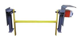
The CTS 700 RBL uses two downcast arms to detect misalignment of a return belt. Should the belt run off to the right or to the left to the extent that it can cause damage to the belt or the conveyor structure, it will come into contact with one of the downcast arms. These arms are connected to an electrical switch via a glass-reinforced polycarbonate made coupling mechanism.
