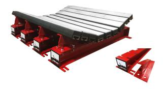
Constructed with more steel than most impact beds, Simplicity Impact Systems provide 75 percent more belt support than conventional impact beds. The impact bars rely on the strength and durability of steel to handle heavy, bulky material, just like the frame. The steel sub-frames in the bars are molded into a shock absorbing rubber and capped with low-friction UHMW, giving your belts a smooth ride out of the loading zone.
