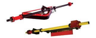
V-Plow discharges material off both sides of the belt while the Angle Plow removes it to one side only. These solutions eliminate uneven buildup on the tail pulley that leads to belt misalignment.
