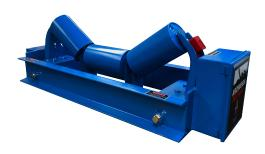
The Archweigh SC offers weight accuracies of 1%-2% as it self-adjusts to the movement of the belt, thanks to Arch's patented dual-ended load cells. This unique engineering compensates for outside forces on the belt by forcing converse reactions by the load cells; one is forced up while the other pushes down. (Constant recalibration is never necessary)
