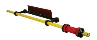
ARCH Saber® Secondary (GSS) cleaners, incorporate the proven Saber® shape into a cantilever style secondary. The patented Twister tensioner applies optimum cleaning pressure to remove carry-back while letting the mechanical splices pass harmlessly, saving the blade, belt, and splice from damage.
