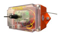
The CTS 300 PSW is a self-wiping rotary switch (not a micro-switch), and consists of two normally open and two normally closed contacts. Once the switch has been tripped, the Blue colored flag is in the "Up" position. The CTS 300 PSW also emits an "Audible" alarm sound before "Start Up" of the conveyor to warn maintenance personnel that the conveyor is about to start.
