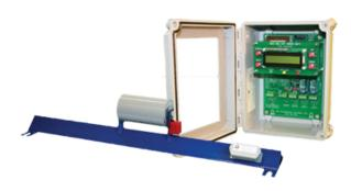
The CTS 700 OSU uses a roller mounted underneath the troughing belt to detect belt movement. A pulse sensor is mounted on the roller structure and monitors the pulses in magnetic proximity mode.
