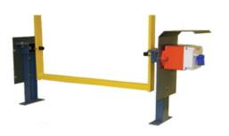
Arch's CTS 700 BL utilizes a mechanical delay to prevent trips from incidental misalignment. The switch features two upright arms connected to a rotary switch that will shut down a conveyor before damage is done. (Once activated, the switch must be manually reset)
