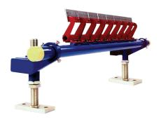
Using metal-bladed technology, the RBS Secondary cleaner eliminates stubborn tack and slime sometimes missed by primary cleaners with a precision-crafted tungsten carbide blade. Delivered pre-assembled to your specifications, this aggressive secondary cleaner is easy to install and handles the toughest conditions at any belt speed.
