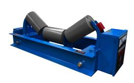
The Archweigh HP is the only belt scale that accounts for outside forces that affect every conveyor. Arch's patented dual-ended load cells mount directly to the idler, and provide reliable, accurate data (up to +/- 1/2%) every day without recalibration. The dual load cells work opposite each other to neutralize the natural lateral and vertical movements of your conveyor belt. As a force pushes down one end, that same force naturally lifts the other; any movement is cancelled out.
