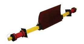
With a HUGE segmented blade pressed on a heavy-duty steel frame and dual Twister® Tensioners, the Super Saber® is the premier defense against stubborn carryback on large belts. Recommended for 30" head pulleys or larger, this is the big solution for big belts.
