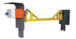
The CTS 700 BTR's two profiled arms connect to a rotary switch equipped with a mechanical delay to prevent trips from incidental contact. (Once activated, the switch must be manually reset)
