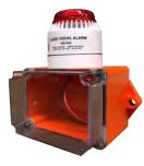
The CTS 900 AVA alarm unit is housed in a high impact UV stabilized polycarbonate enclosure rated to IP 65 degrees of protection. The unit consists of: 1 alarm buzzer rated 105 dB and a flashing strobe light.
