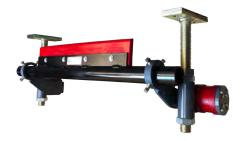
The RGS secondary utilizes a Heavy-duty trailing arm frame supported by 1½ inch spindles. An internal Twister Tensioner maintains the constant pressure of a urethane encased, tungsten carbide blade. This tough combination makes easy work of any residual material missed by a primary cleaner.
