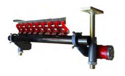
Using metal-bladed technology, the RBS Secondary cleaner eliminates stubborn tack and slime sometimes missed by primary cleaners with a precision-crafted tungsten carbide blade. Delivered pre-assembled to your specifications, this aggressive secondary cleaner is easy to install and handles the toughest conditions at any belt speed.
