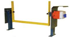
Arch's CTS 700 BL utilizes a mechanical delay to prevent trips from incidental misalignment. The switch features two upright arms connected to a rotary switch that will shut down a conveyor before damage is done. (Once activated, the switch must be manually reset)
