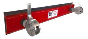
Utilizing a cam action, the Cam-A-Lot Clamp System makes quick work of changing skirtboard rubber. 360 degree rotating clamp heads allow for a custom fit in an otherwise unusable space. Simple and easy weld on installation makes the Cam-A-Lot a hassle free solution to load zone sealing.
