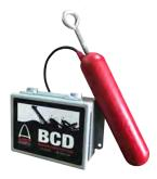
The CTS 600 BCD blocked chute detector is a tilt-type switch, which is mounted inside the chute to monitor any blockage in the material conveyed. Should material start to build up due to a blockage, it will lift the sensing rod, tilting the switch; any tilt to the switch above 15 degrees will cause one of the steel-encapsulated switches to open. This unit provides a relay interface between a tilt-type probe and the conveyor control system.
