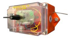
The CTS 300 PSW is a self-wiping rotary switch (not a micro-switch), and consists of two normally open and two normally closed contacts. Once the switch has been tripped, the Blue colored flag is in the "Up" position. The CTS 300 PSW also emits an "Audible" alarm sound before "Start Up" of the conveyor to warn maintenance personnel that the conveyor is about to start.
