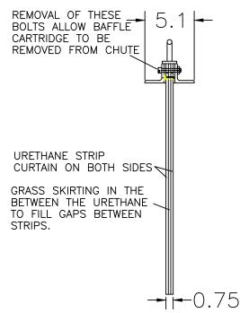
CHUTE BAFFLES ARE MADE TO ORDER BASED ON WIDTH REQUIRED FOR THE APPLICATION. WHEN ORDERING PLEASE SPECIFY DIMENSION "X" IN THE DIAGRAM ABOVE
