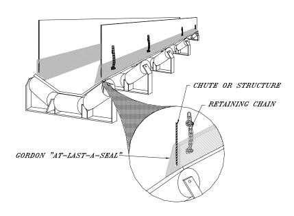
Note: A good quality rubber lubricant applied to the inside of the skirt rubber will make the installation much easier.
