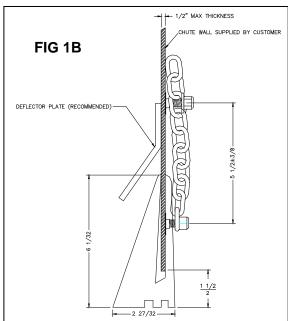
These dimensions will allow the skirt rubber to "float" with the belt and makes it much easier to slide the skirt rubber onto the chute wall. Leave 6 inches of skirt rubber extending past the backside of the chute (Fig 2 – Dimension 'C').
